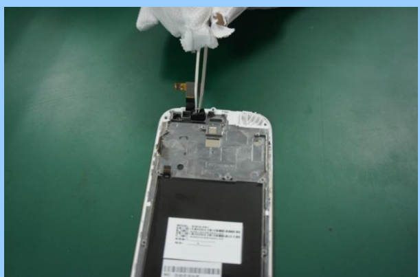
Remove the induction gum cover.....9
