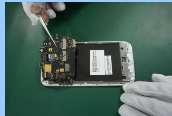
Install the PCBA.....4
