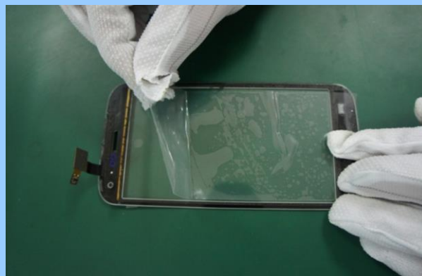
Tear off protection film.....2
