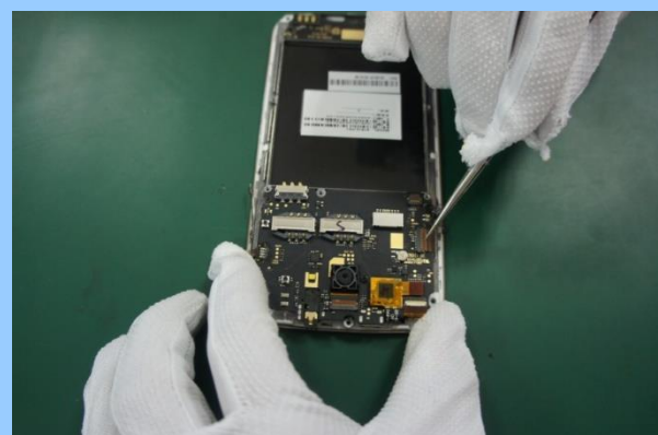
Remove the LCD FPC.....5
