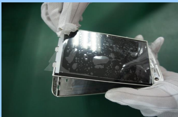
Remove the LCD.....15
