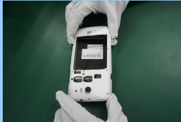
Install the back cover .....12
