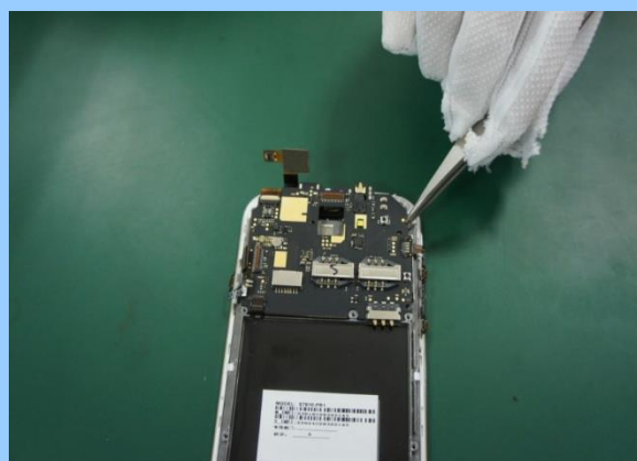
Remove the PCBA.....8
